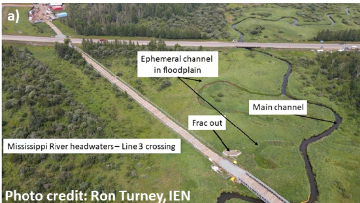
Figure 2. a) Top photo shows location of first known frac out at Mississippi River Crossing #1, observed by water protectors in a wetland on July 20, 2021. b) Right photo shows Enbridge workers attempting to clean up drilling fluid spill in the same wetland.
